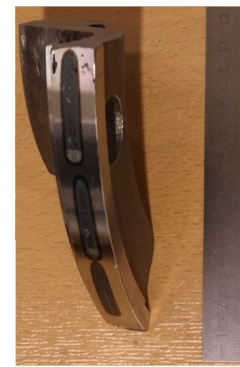
Fig. 7. Fragment of a steel C45 part with a laser track on the surface
